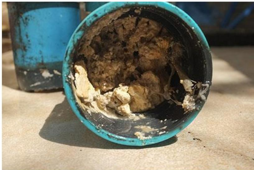
Photo courtesy of: [quickerrooterplumbing.ca](http://quickerrooterplumbing.ca)
